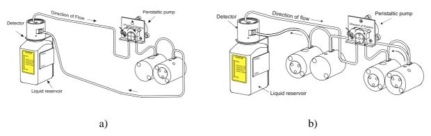
Fig. 23: Active rear-seal wash system (connection) a) for a P680A ISO and P680A LPG-4 b) for a P680A HPG-2, P680A HPG-4, P680A DGP-6, and P680P HPG-2
