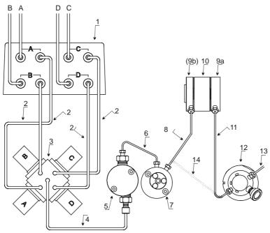
Fig. 34: Connections for a low-pressure gradient system
