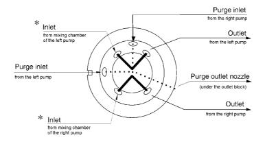
Fig. 30: Outlet block (for P680A DGP-6 pumps)
