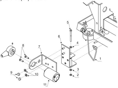
Fig. 40: Installing the manual injection valve
