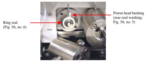
Fig. 59: Pump head removed
