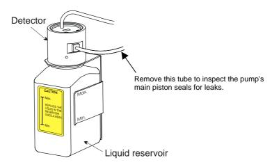
Fig. 57: Liquid reservoir of the rear-seal wash system
