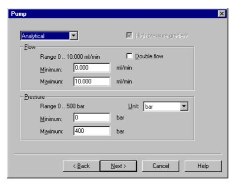
Fig. 51: Pump wizard page (here: for P680 HPG pumps)
