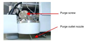
Fig. 26: Purge block for all P680 pump types except P680A DGP-6
