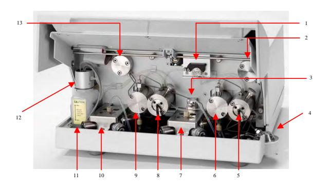
Fig. 35: Open P680A DGP-6 pump (view from front)
