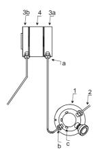
Fig. 65: Connections between mixing chamber and purge block (all pumps except P680A DGP-6)
