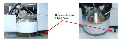
Fig. 3: Waste outlet (left: all P680 pumps except P680A DGP-6; right: P680A DGP-6)
