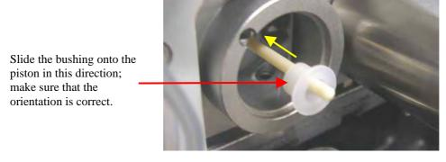
Fig. 63: Correct orientation of the bushing with draining device
