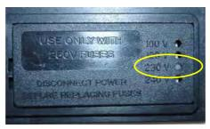
Fig. 4: Factory-set voltage selection, here: 230V
