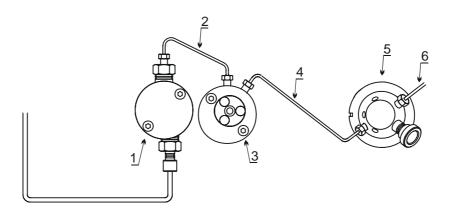
Fig. 32: Connections for an isocratic pump system
