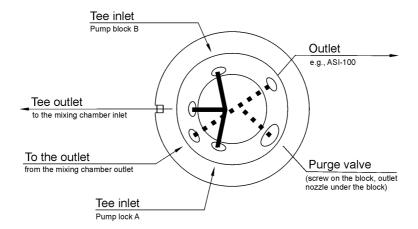
Fig. 29: Purge block (except for P680A DGP-6 pumps)
