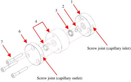
Fig. 64: Mixing chamber with optional mixing chamber extension
