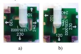
Fig. 7: Voltage selector board settings a) for 200V-240V and b) for 90V-130V
