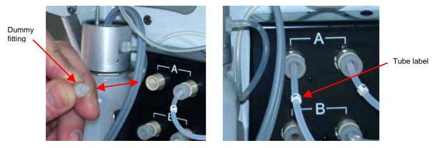
Fig. 15: Connecting the solvent reservoir (P680A LPG-4 pump)
