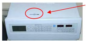
For P680A ISO, P680A HPG-2, P680A HPG-4, and P680A DGP-6 pumps, the solvent lines are already installed at the factory and routed through this opening in the top cover.
