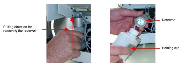
Fig. 24: Liquid reservoir of the rear-seal wash system
