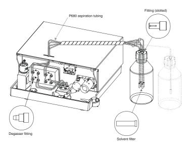
Fig. 16: P680A LPG-4 pump with solvent rack connection
