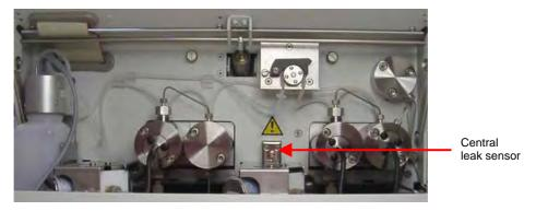
Fig. 55: Central leak sensor (here: P680 HPG)
