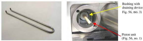
Fig. 60: Extractor for bushing with draining device
