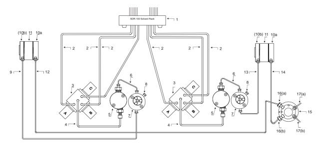
Fig. 36: Connections for a dual low-pressure gradient system
