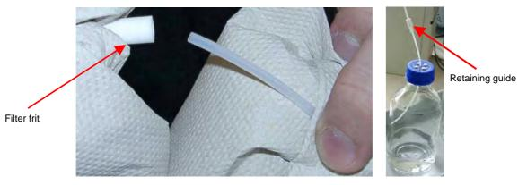
Fig. 13: Connecting the solvent lines to the reservoir
