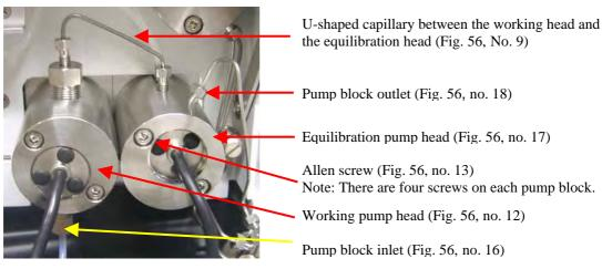
Fig. 58: Installed pump heads
