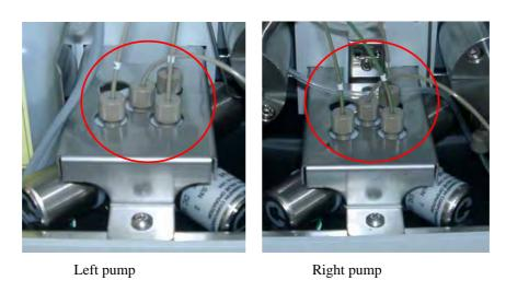
Fig. 17: Connecting the solvent lines (P680A DGP-6 pump)
